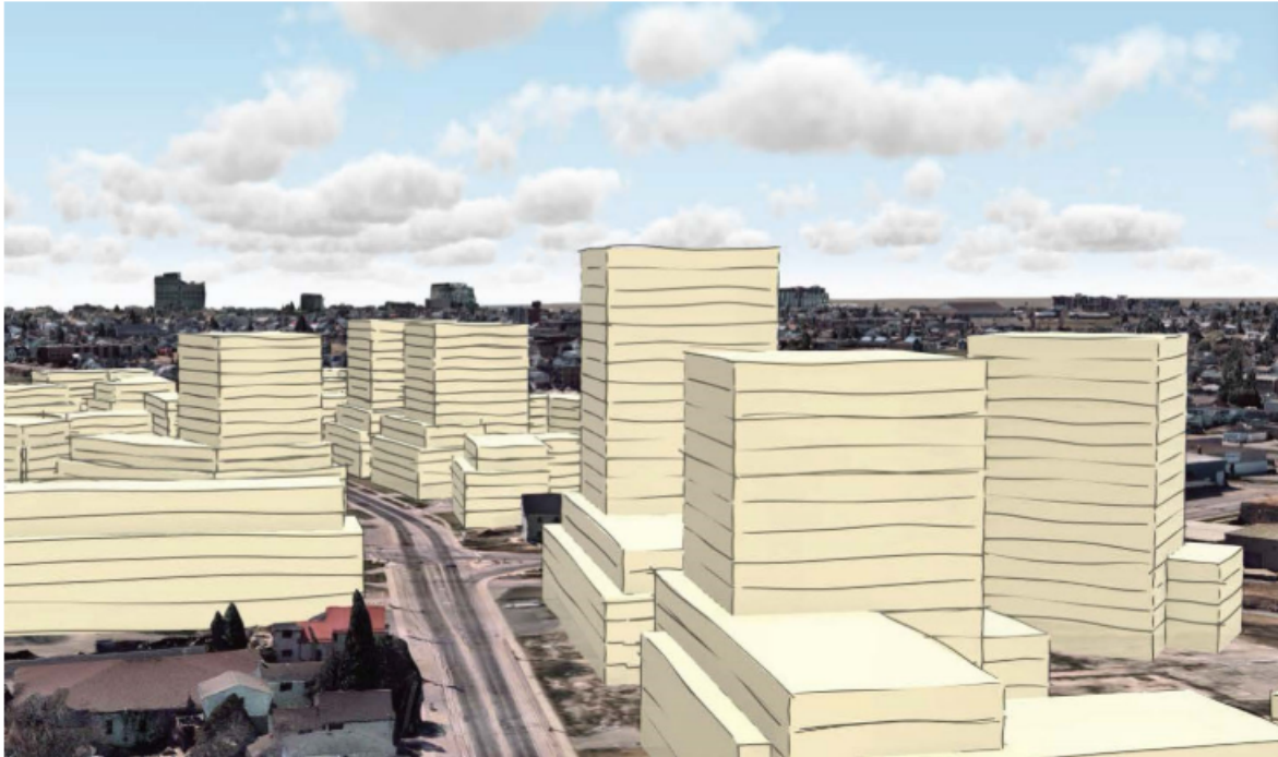
Figure 3 – Aerial view looking south along Montreal Street, near the intersection with Rideau Street and Railway Street showing conceptual massing within intensification areas and use of building setbacks and stepbacks.
