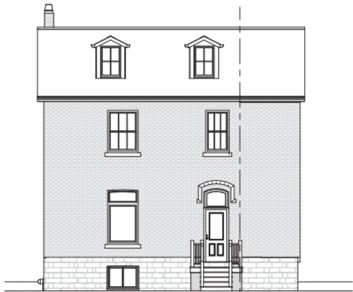
North Elevation (Existing)
