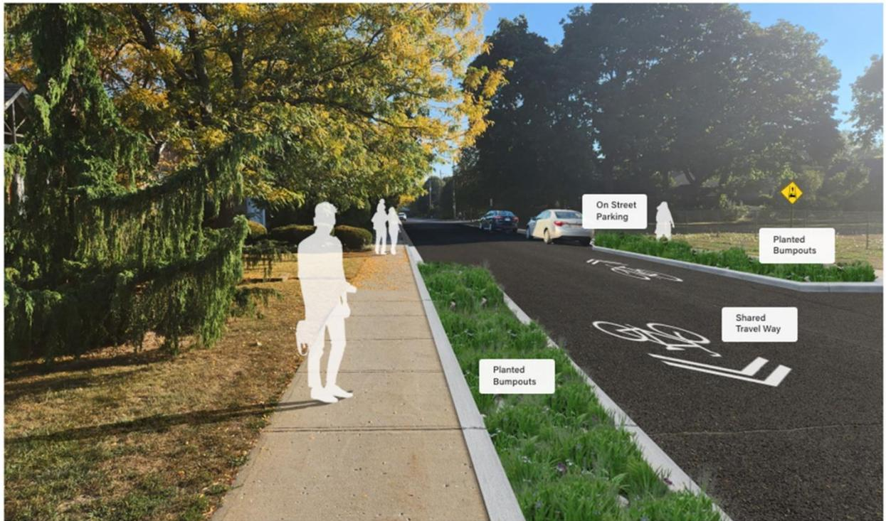
Figure 17: Typical 20 Metre Right-of-way Neighbourhood Bikeway
