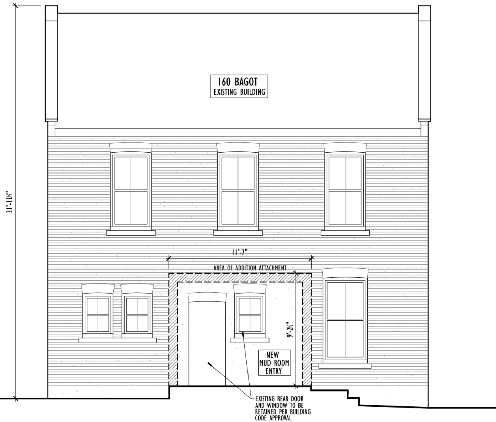
REAR ELEVATION - EXISTING BUILDING 0 1 2 4 FT
