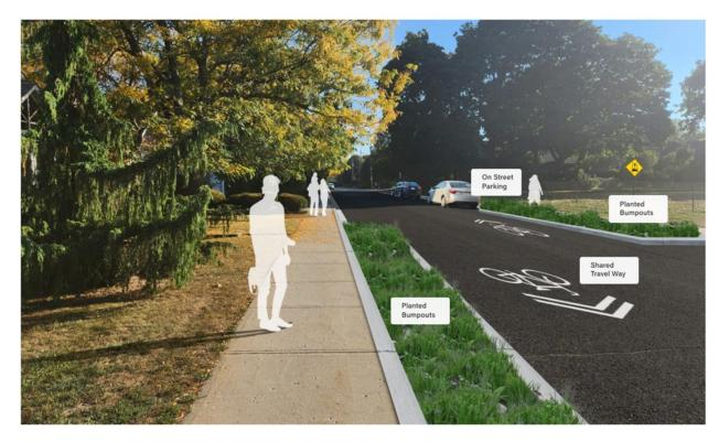
Figure 16: Typical 15 Metre Right-of-way Neighbourhood Bikeway
